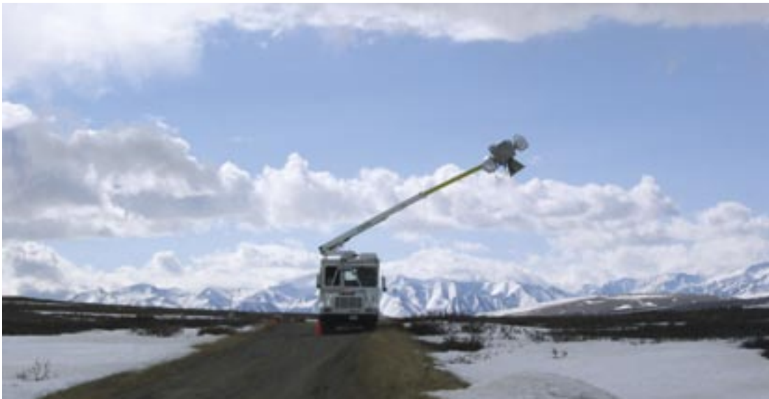
Radiometers on the boom of the truck viewing the Arctic shrub site to the west side of the lane. On the east side of the lane is the micrometeorological station at the nearby tussock tundra site. Brooks Range is in the background.
